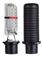
FOSC® 450 D6 Fiber Optic Splice Closure, Gel Cable sealing, one preinstalled 36-splice tray, 4 cable attach., three ground feedthrough lugs, with test valve
