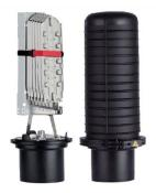
FOSC® 450 B6 Fiber Optic Splice Closure, Gel Cable sealing, no preinstalled trays, 4 cable attach., three ground feedthrough lugs, with test valve
