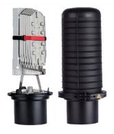
FOSC® 450 A4 Fiber Optic Splice Closure, Gel Cable sealing, one preinstalled 24-splice tray, 4 cable attach., one ground feedthrough lug, with test valve
