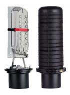
FOSC® 450 D6 Fiber Optic Splice Closure, Gel Cable sealing, one pre-installed 72-splice tray, 6 cable attach., three ground feedthrough lugs, with test valve
