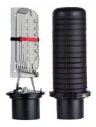
FOSC® 450 D6 Fiber Optic Splice Closure, Gel Cable sealing, one preinstalled 72-splice tray, 6 cable attach., six ground feedthrough lugs, with test valve
