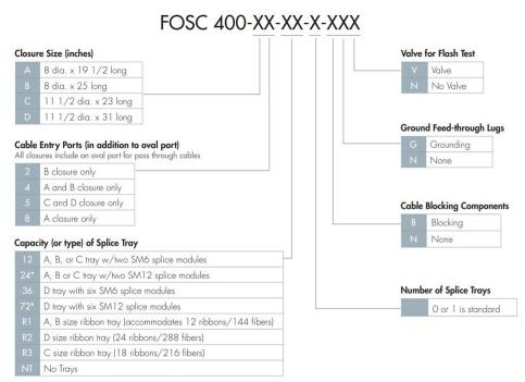
\*Note: SMOUV (1120-01-US) splice protection sleeves should be used with SM12 splice modules.
