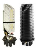
FOSC® 400 D5 Fiber Optic Splice Closure, Heat Shrink Cable sealing, two pre-installed 36-splice trays, cable blocking, ground feedthrough lugs, with test valve
