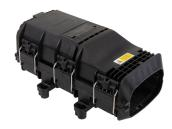
OFDC B8G Fiber Optic Splice/Patch Closure, Gel Cable sealing, 4 pre-installed 12-fiber splice trays, 1 pre-installed 18-fiber splice tray, 8 SC/APC adapters and pigtails
