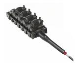
DLX® Mini-MST, Fiber Optic Multiport Service Terminal, 8-port with 1x8 splitter, dielect. flat loose tube cable, Hardened mini-size DLX connector on stub end, 100 m
