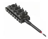
DLX® Mini-MST, Fiber Optic Multiport Service Terminal, 8-port with 1x8 splitter, dielect. flat loose tube cable stub, unterminated, 150 ft
