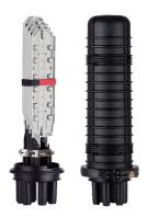
FOSC® 450/B Fiber Optic Splice Closure, Gel Cable sealing, with integrated DWDM, 8 channels + upgrade port, double demux, 2 test ports
