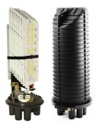
FOSC® 400 D5 Fiber Optic Splice Closure, Heat Shrink Cable sealing, six pre-installed 24-fiber trays
