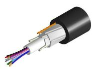
Fiber Indoor/Outdoor Drop Cable, LazrSPEED®, Low Smoke Zero Halogen Single Jacket All-Dielectric Arid-Core, 6 fiber, Gel-filled, Multimode OM3, Feet jacket marking, Black jacket color, Dca flame rating
