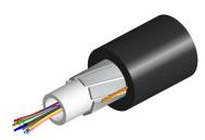
Fiber Indoor/Outdoor Drop Cable, TeraSPEED®, Low Smoke Zero Halogen Single Jacket All-Dielectric Arid-Core, 12 fiber, Gel-filled, Singlemode + Multimode OM3, Feet jacket marking, Black jacket color, Dca flame rating
