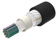
Fiber indoor/outdoor cable, All-Dielectric, LSZH Riser-Rated, Gel-Free, Central Tube Rollable Ribbon, 432 fiber, Singlemode G.652.D and G.657. Al, Feet jacket marking, Black jacket color, Cca flame rating
