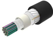
Fiber indoor/outdoor cable, All-Dielectric, LSZH Riser-Rated, 144 fiber, Gel-Free, Central Tube Rollable Ribbon, Singlemode G.657.A2/B2, Feet jacket marking, Black jacket color, Cca flame rating
