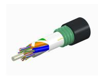
Fiber indoor/outdoor cable, TeraSPEED®, Single Jacket/Single Armor, Low Smoke Zero Halogen (LSZH), 48 fiber, Singlemode G.652.D and G. 657.A1, Gel-Free, Stranded Loose Tube, Black jacket color, Meters jacket marking
