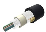
Fiber OSP Cable, Non-Armored, All-Dielectric, 216 fiber, Arid-Core, Dry Central Tube Ribbon, Multimode OM3 bend insensitive, Gel-free, Feet jacket marking, Black jacket color
