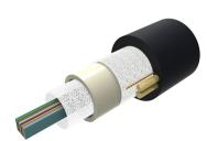
Fiber OSP Cable, Non-Armored, All-Dielectric, Arid-Core, 36 fibers, Dry Central Tube Ribbon, Multimode OM3 bend insensitive, Gel-free, Feet jacket marking, Black jacket color
