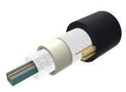
Fiber OSP Cable, Non-Armored, All-Dielectric, Arid-Core, 216 fiber, Dry Central Tube Ribbon, Singlemode G.652.D and G.657.Al, Gel-free, Feet jacket marking, Black jacket color
