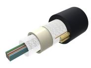
Fiber indoor/outdoor Cable, LSZH Riser All-Dielectric Central Tube Ribbon, Multimode OM4 bend insensitive, 12-fiber, feet jacket marking, black jacket color
