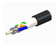
Fiber OSP cable, TeraSPEED® Single Jacket All-Dielectric, 48 fiber, Gel-Free, Outdoor Stranded Loose Tube w/HDPE Outer Jacket, Singlemode G.652.D and G.657.Al, Feet jacket marking, Black jacket color
