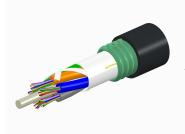
Fiber OSP cable, TeraSPEED® Single Jacket/Single Armor, 120 fiber, Gel-Free, Stranded Loose Tube, Singlemode G.652.D and G.657.A1, Feet jacket marking, Black jacket color
