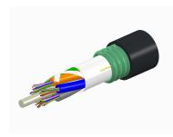
Fiber OSP cable, TeraSPEED® Single Jacket/Single Armor, Gel-Free, 48 fibers, Stranded Loose Tube, Composite OM4 and G.652.D and G.657.A1, Feet jacket marking, Black jacket color
