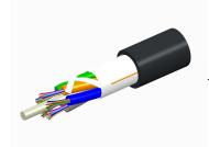
Fiber OSP cable, TeraSPEED® Single Jacket All-Dielectric, 216 fiber, Gel-Free, Stranded Loose Tube, Singlemode G.652.D and G.657.A1, Feet jacket marking, Black jacket color
