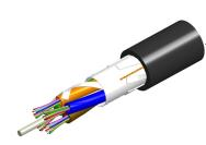
Fiber OSP cable, LazrSPEED®, Light Duty, Single Jacket, All-Dielectric, 6 fiber, Gel-Free, Stranded Loose Tube, Multimode OM3, Feet jacket marking, Black jacket color
