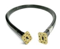
FlexTwist® Flexible Twist for WR75, 10.0–15.0 GHz, with interface types PDR120 and PBR120, 600 mm
