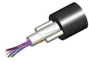
Fiber Indoor/Outdoor cable, Single Jacket Gel-Filled All-Dielectric, 36 fibers, Riser Rated Central Tube, Singlemode G.657.A2/B2, Feet jacket marking, Black jacket color
