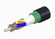
Fiber indoor/outdoor cable, LazrSPEED®, Single Jacket/Single Armor, Low Smoke Zero Halogen (LSZH), Gel-Free, 144 fiber, Stranded Loose Tube, Multimode OM3, Black jacket color, Feet jacket marking
