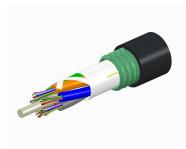
Fiber indoor/outdoor cable, LazrSPEED®, Single Jacket/Single Armor, Low Smoke Zero Halogen (LSZH), 24 fiber, Gel-Free, Stranded Loose Tube, Multimode OM3, Black jacket color, Feet jacket marking
