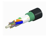
Fiber indoor/outdoor cable, TeraSPEED®, Single Jacket/Single Armor, Low Smoke Zero Halogen (LSZH), 144 fiber, Singlemode G.652.D and G. 657.A1, Gel-Free, Stranded Loose Tube, Black jacket color, Feet jacket marking
