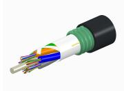
Fiber indoor/outdoor cable, TeraSPEED®, Single Jacket/Single Armor, Low Smoke Zero Halogen (LSZH), 96 fiber, Singlemode G.652.D and G. 657.A1, Gel-Free, Stranded Loose Tube, Black jacket color, Feet jacket marking
