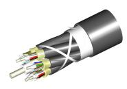
Fiber Indoor/Outdoor cable, TeraSPEED® Low Smoke Zero Halogen Riser Distribution, 36 fiber multi-unit with 12 fiber subunits, Gel-free, Singlemode + Multimode OM4, Feet jacket marking, Black jacket color, Cca flame rating
