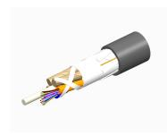
Fiber indoor/outdoor cable, TeraSPEED®, Single Jacket All-Dielectric, Plenum Rated, Multimode/Singlemode, 36 fiber, Gel-Free, Stranded Loose Tube, PVDF jacket, Black jacket color, Feet cable marking
