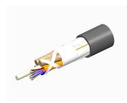
Fiber indoor/outdoor cable, TeraSPEED®, Single Jacket All-Dielectric, Plenum Rated, Multimode/Singlemode, 24 fiber, Gel-Free, Stranded Loose Tube, PVDF jacket, Black jacket color, Feet cable marking
