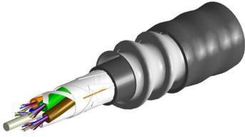
Fiber indoor/outdoor cable, TeraSPEED® Inner LSZH, 48 fiber, Mini Stranded Loose Tube, Riser Rated, Singlemode G.652.D and G.657.A1, Gel-Filled Subunits, Aluminum Interlocking Armor, Feet jacket marking, Black jacket color
