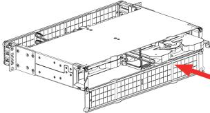
Once the cassette is inserted into the panel, the door can be closed by rotating it back into place until the two latches on each side click into position.
