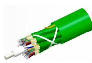
Fiber indoor cable, TeraSPEED® Plenum Distribution, 48 fiber multi-unit with 12 fiber subunits, Singlemode G.652.D and G.657.A1, Gel-free, Feet jacket marking, Green jacket color
