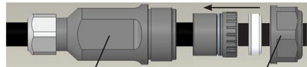
M40 spanner M42 spanner (Torque force: 2.5 N·m)
