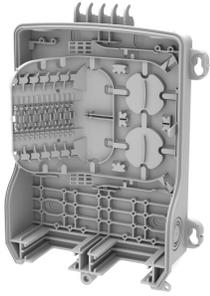
IFEB20, Indoor Fiber Optic Wall mount Enclosure, Splice Only, Single Element Slim trays(12) Smouv, Feeder cable seal 2x15 and 16x7mm drop seal, RAL 9010
