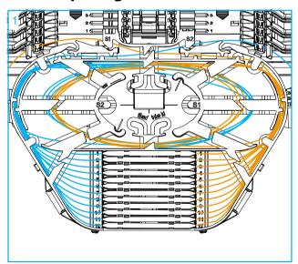
1 Make splice per local practice and store the splice protector in the splice protector holder. Store the over lengths in loops in the over length storage area.
