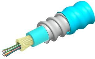
Fiber indoor cable, LazrSPEED® Plenum Distribution, interlocking aluminum armored with plenum jacket, 24 fiber single-unit, Gel-free, Multimode OM4, Feet jacket marking, Aqua jacket color
