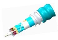
Fiber indoor cable, LazrSPEED® Riser/LSZH rated, Distribution, interlocking aluminum armored, Multimode OM3, 72 fiber multi-unit with 12 fiber subunits, Gel-free, Feet jacket marking, Agua jacket color
