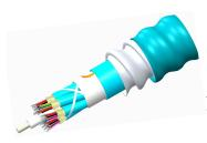
Fiber indoor cable, LazrSPEED® Riser/LSZH rated, Distribution, interlocking aluminum armored, Multimode OM3, 36 fiber multi-unit with 12 fiber subunits, Gel-free, Feet jacket marking, Aqua jacket color
