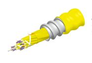
Fiber indoor cable, TeraSPEED® Plenum MPO Trunk, interlocking aluminum armored with plenum jacket, Singlemode G.652.D and G.657.A, 36 fiber multi-unit with 12 fiber subunits, Yellow jacket color, Feet cable marking
