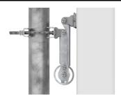
Wide Profile Antenna Downtilt Mounting Kit for 2.4 - 4.5 in (60 - 115 mm) OD round members. Kit contains one scissor top bracket set and one bottom bracket set.
