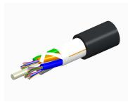
Fiber OSP cable, LazrSPEED® Single Jacket All-Dielectric, Gel-Free, 2 fiber, Stranded Loose Tube, Multimode OM3, Feet jacket marking, Black jacket color
